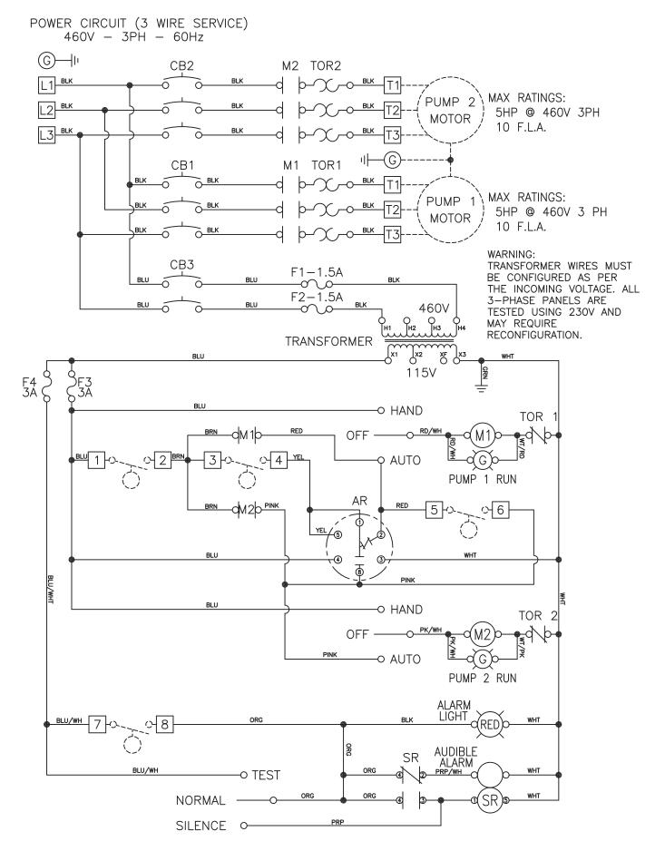
NOTES: FLOAT SWITCH TO BE RATED 2 AMPS @ 120V MINIMUM. MAIN PANEL DISCONNECT MUST BE PROVIDED BY INSTALLER. DASHED LINES INDICATE ITEM NOT CONTAINED IN THE PANEL. FIELD WIRING MUST BE A MINIMUM OF 60° COPPER WIRE.
