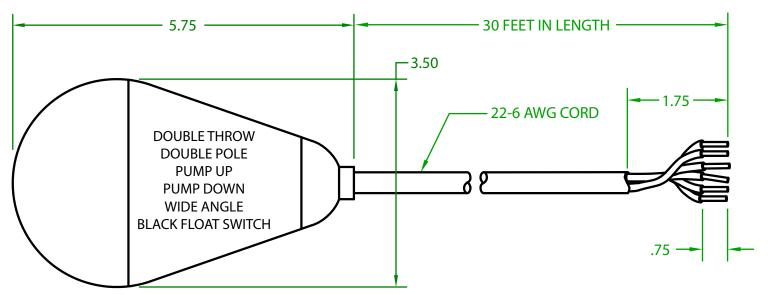
OPERATING ANGLE: FLOAT HANGING DOWN CONTACTS ARE OPEN CONTACTS CLOSED @ 45° ABOVE HORIZONTAL CONTACTS OPEN @ 45° BELOW HORIZONTAL
